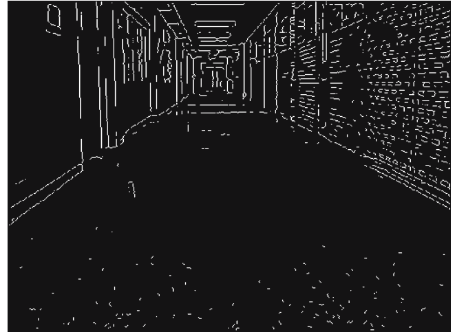
Fig. 7 Edge detection using higher-order neural units
